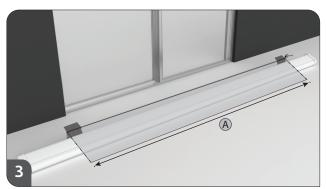
Insert the wall brackets (nº8) in casing holders (nº4) and measure it (A) with the supports. Transport this measure (A) to the ceiling where it will fixed. From here, follow all the steps used in the wall installation (page 03.B) using, in this case, the brackets (nº21) for the safe fixation in the area B of the image 1.
