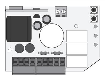
Control board MC6, for awning automation, with possibility to connect a presence light with timer, with operation via transmitter and Wireless Sensor (sun/wind/rain).
