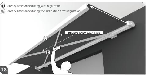
**o1** - To start the inclination arms regulation, fully open the awning. Assist the awning indicated area during the whole regulation process (E).
