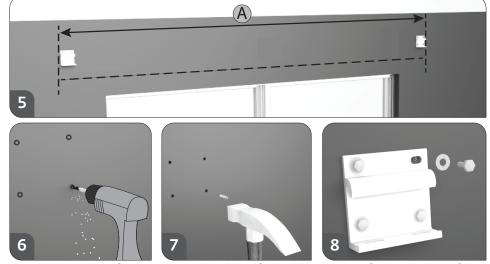
$o_3$  - With the help of a pencil or marker, identify the drilling points for the placing of the wall brackets ( $n^28$ ). Make holes with 100mm deep and  $\varnothing$ 20mm.
