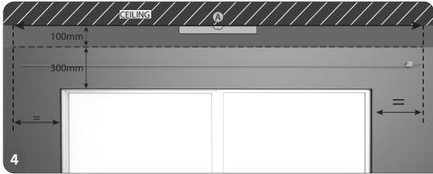
**o2** - Take the measurement at the location where the awning will be applied. Pay attention to the leveling of wall brackets (**nº8**) for fixing the awning.
