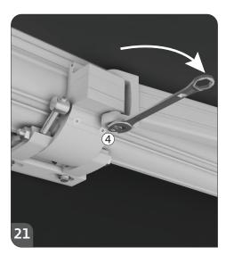
**o1**-With the awning open for about 500 mm, loosen the nut ⓐ approximately 7mm so that the upper part of screw is loosened out of the arm.
