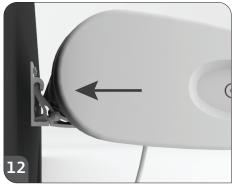
**o5** - Make the application of the awning, fitting casing holders (**nº4**) in the wall bracket (**nº8**). Please check the images **9**, **10**, **11** and **12**.
