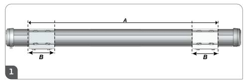
For a correct operation of the awning, the measure **A** can not be changed. The wall bracket (**n° 8**) must be placed in zone **B** where the casing support (**n° 4**) is.
