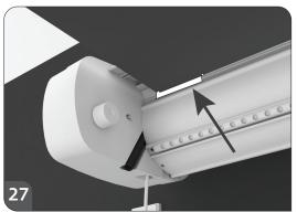
If you detect any anomalies in the fabric winding (total closure of a side only), make the opening of the awning and place plastic shims in the place identified in the **image 27** (the side that does not close).
