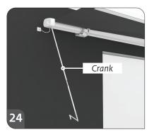
The awning is prepared for, in case of power failure or other situation that prevents the electrical operation of the equipment, it is possible to make the opening or closing manually by using the handle (nº20).
