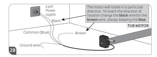
To detect possible problems in the motor, it will be necessary to conduct tests with direct connection to a 230V power supply.
