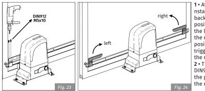
1 • After having rack nstalled, take the gate back to the closed position and position the limit swicth plate on the rack. In this closed position, the plate should trigger the limit switch of the motor.
