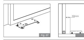
Fit the 4 supplied nuts, as shown in Fig. 07 and Fig. 08, in the 4 holes of the plate.
