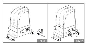
Insert supplied key on the lock, turn it clockwise 90° (Fig.18), pull and open the manual release (Fig.19).
