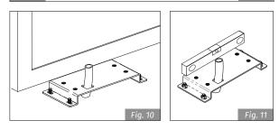
2 • Put the foundation plate to the floor, using adequate expansion plugs and provide one or more tubes for routing the electric cables through the plate (Fig10 and 11).
