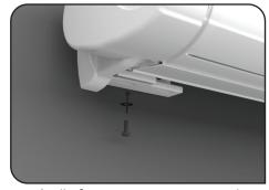
**12** - Finally, fasten one M10 screw on the wall brackets to secure the awning.
