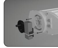
**o2** - Remove the control board and the transformer.
