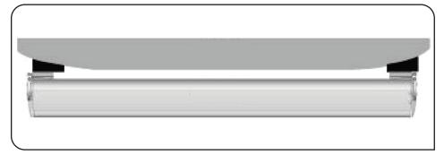
Before starting the installation, check the leveling of the wall. If the wall is hollow or curved, please calibrate the wall with the help of a support in order to properly align the fastening points (refer to above image).
