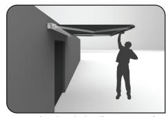
**o3** - During the whole adjustment, assist by hand the front of the awning to relieve the weight on the pin.
