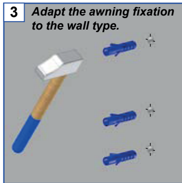
Fixation with Ø12mm screws. Screws Kit, anchors and washers are not included/provided.
