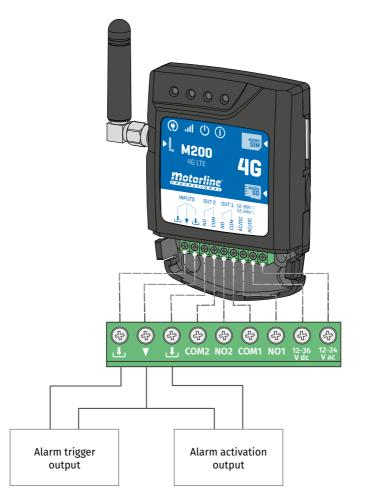
As soon as the alarm is triggered, Input 2 is activated and the system starts making calls to the contact list in order of listing until a contact answers.
