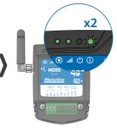
3 • Wait until the ACT LED starts flashing 4 times with 1 second interval;
